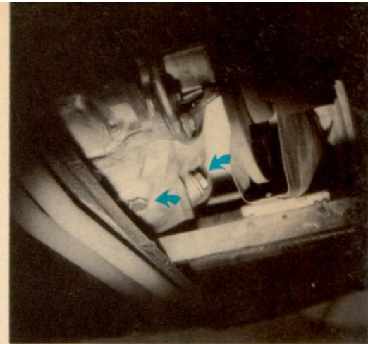
Transmission-differential; Oil-level, and Drain Plugs. Check every 3600 miles. Change every 12,000 miles.
