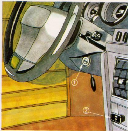
Fig. 10 - Starting 1 - Combined anti-theft-ignition-starting switch 2 - Choke control
