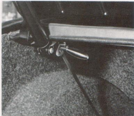
Fig. 31 - Inserting the locking pin on the rear height adjustor
