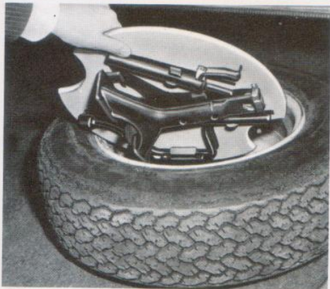
Fig. 28 - Tools for removing the wheels
