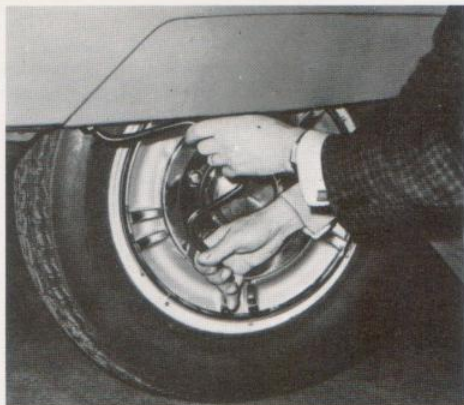
Fig. 30 - Removing the fender skirt
