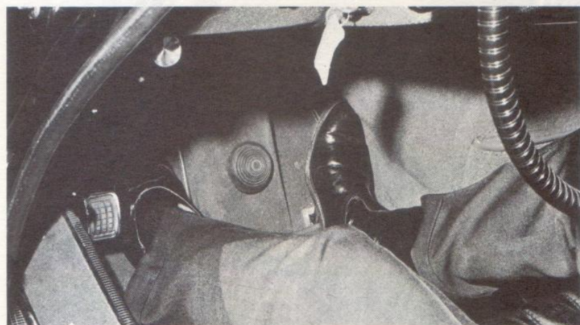
Button that looks like a headlight beam switch is the Citroën brake pedal. Parking brake release is a little awkward in use.
