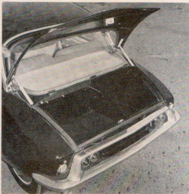
Though short, the bed is amply comfortable for a night's rest. Painted windowsills and door latch-lock-grab bar, with extensive use of plastic, do not carry out the car's luxury feel. Trunk floor is the belly pan.
