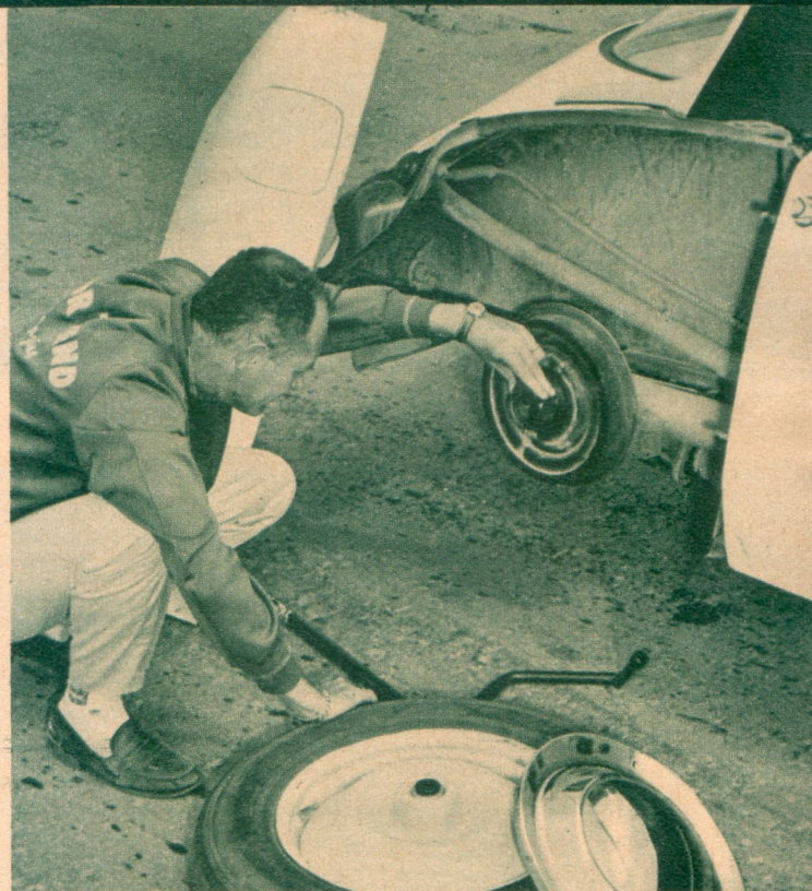
WHEEL CHANGE is accomplished by removing two bolts: one from fender, one from wheel.
